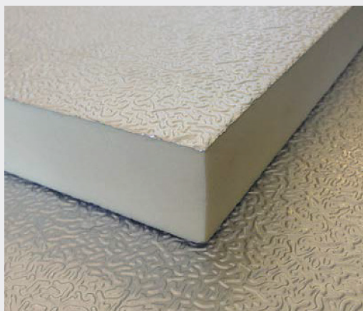
Figure 2: a) PIR board insulation with foil facers (photo courtesy of Pirmax Pty Ltd), b) Installation of polyurethane spray foam to a wall (photo courtesy of Huntsman International LLC).
