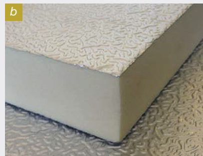
Figure 1: a) Schematic illustration of the continuous insulation concept for a timber frame wall, b) PIR board insulation with foil facers (photo courtesy of Pirmax Pty Ltd).
